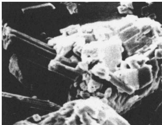
Figure 1. Aged TPA particle ( \times 820 ) after 60 min at 480 K in a glass capillary.
